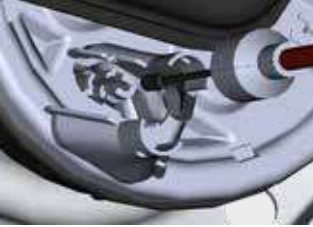
Hook-in Bowden cable saves assembly time.
