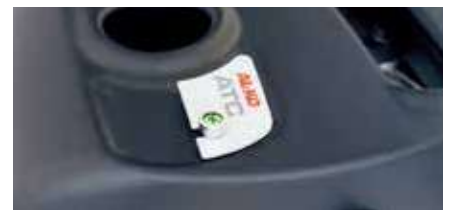
The LED on the overrun device lights up green. The system is 100% functional.
