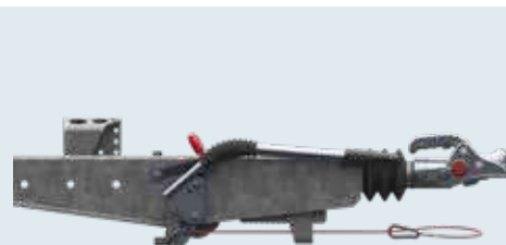
Handbrake lever opened = brake rod not clamped
