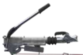
Handbrake lever closed (parking brake forwards)
