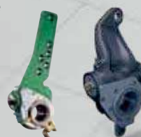
Brake adjusters AA1, S-ABA
