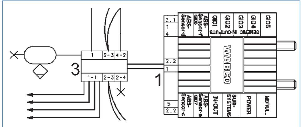
In the absence of a PEM, overload protection must be ensured using a separate relay overload protection valve:
