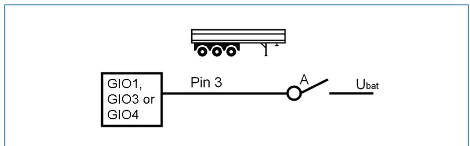
Mechanical switch IV for road finishers to positive at digital TEBS E input (resistance cable not supplied by WABCO)
