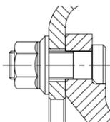
\* According to DIN 74361 part 3 strength class of 10 respectively 10.9 according to ISO 898 is necessary for the nut and for the bolt.
