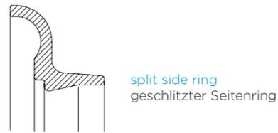
For reason of safety it is of vital importance to use the correct pertinent split side ring (combination ring). It is recommended to assemble the separation gap of the split side ring twisted by at least 45° relation to the valve slot.
