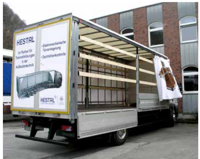
For example: HESTAL MaxiKit curtainsider superstructure with Hestal Snap dropsides and SmartMaster rear door
