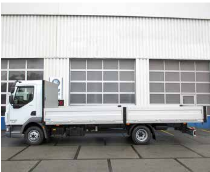
For example: HESTAL flatbed superstructure with elevated HESTAL Snap front wall
