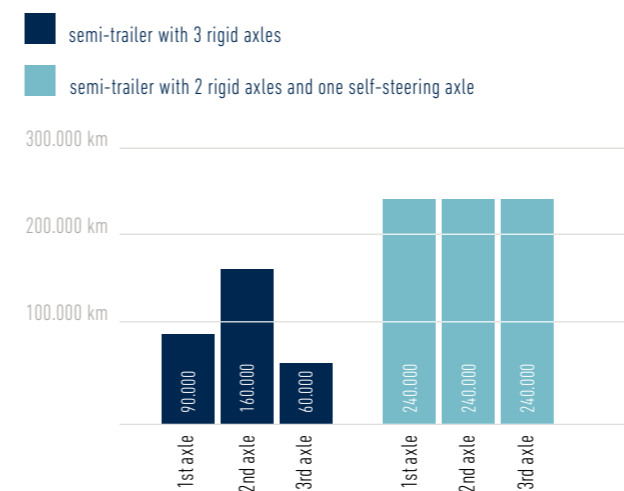
service life of wheels in km during distribution transport
