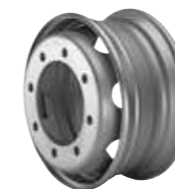
alive DISC WHEEL FOR DUAL FITMENT WITH 15° DROP CENTRE RIM FOR TUBELESS TYRES
