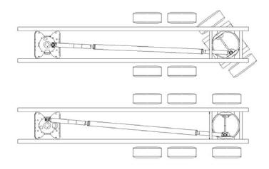
The TRIDEC TD steering system is a mechanical steering system used primarily in distribution transport. This system steers one axle of a one, two or three-axle trailer, but it can also steer two axles.
