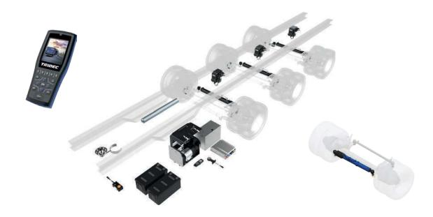
TRIDEC's EF-S steering system enables trailers with an extremely low trailer neck, such as milk and bulk tankers or trailers with monocoque-constructions, to be equipped with a steering system for kingpin axles. Because of the weight advantage, as well as the minimal required mounting space and easy installation, the system can also be applied to low-loaders.
